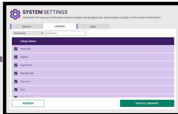
Figure 25. Analyte management to view or hide analytes available in Analyze mode
