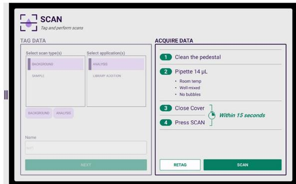
Figure 10. For optimal results, follow steps 1-4 to acquire scan data.
