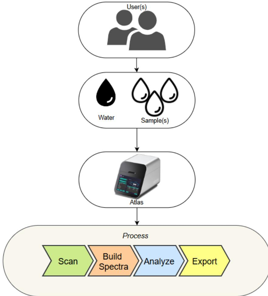
**Figure 6.** Overview of the user workflow for sample analysis with Atlas.
